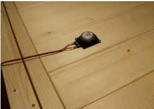
Fig. 47: Installation of the exciter
