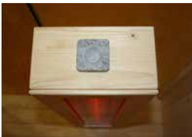
Fig. 31: Inserting the soapstone bowls
